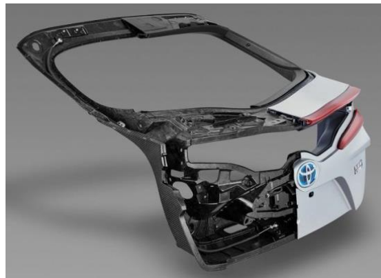
Figure 1-3: PHV hybrid vehicle carbon fibre SMC door frame [35]
