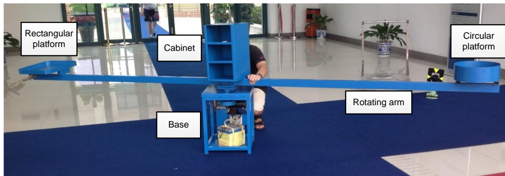
Figure 7. The rotating arm rig for testing of the proposed method with real multipath data.
