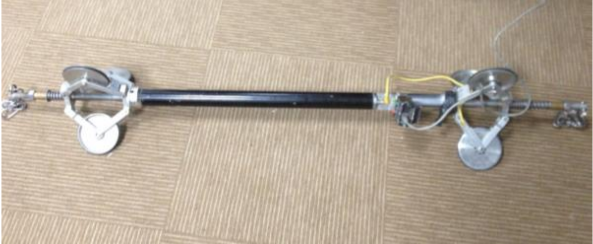
Figure 3 Ductrunner consisting of a probe and two wheel sets.
