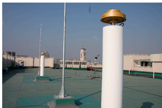
Figure 3. GNSS reference stations in UNNC.
