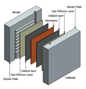
**Figure 2.** Schematic of a single-cell PEM fuel cell with straight channels.
