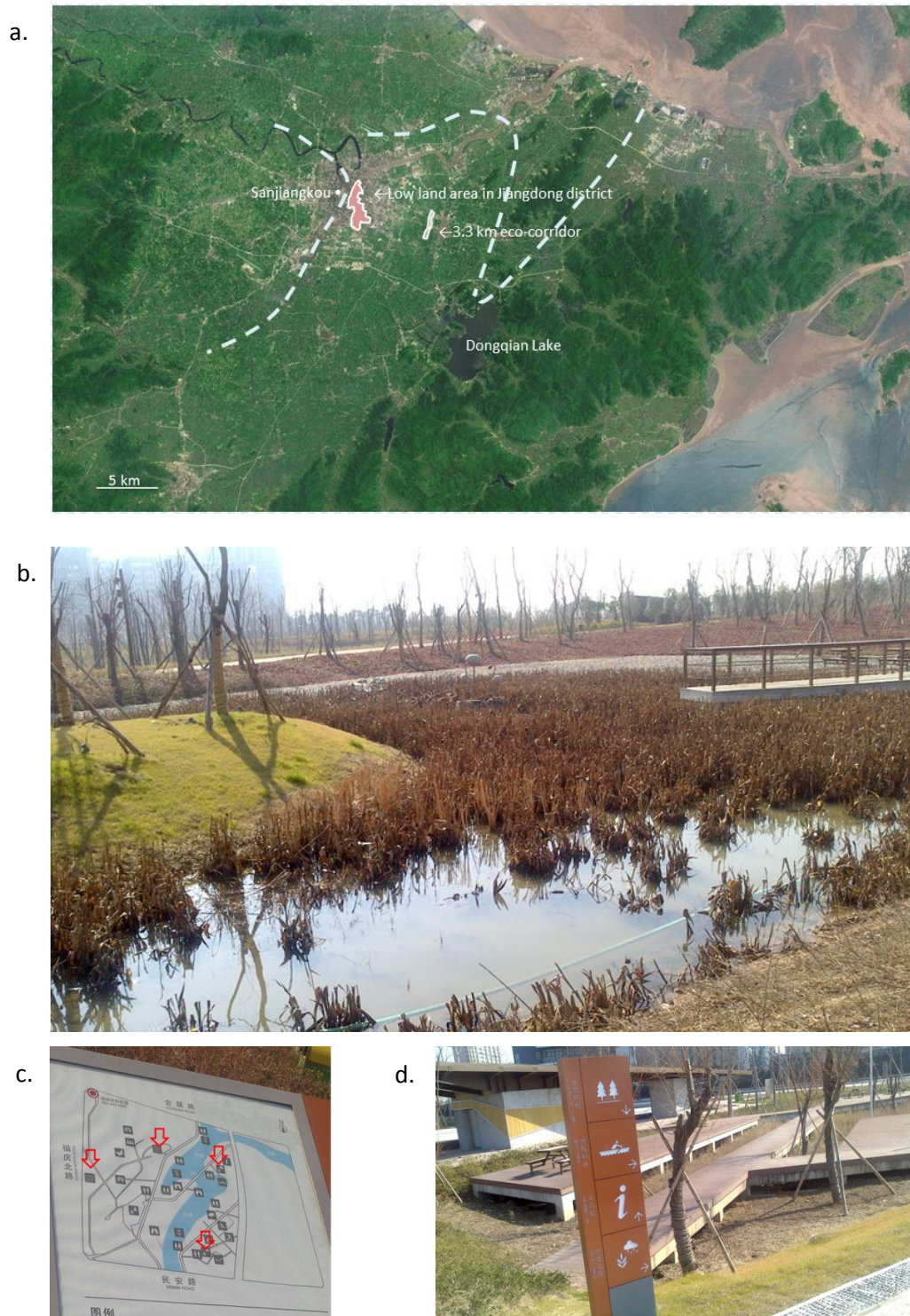
Fig. 7. Planned and Established Eco-corridor in Ningbo Area. a. relative scale and locations of the 3.3 km exemplary eco-corridor (white block), the three planned eco-corridor with the function of 5 to 10 km width greenbelt of the city (dash lines) and the areas seriously affected by the flood in the city centre (pink shading area). b. A recreated marshland area in the established part of the eco-corridor. Source: Picture Taken by Authors. c. The map installed in one section of the new Eco-corridor. The red arrows indicated the locations of water retention facilities for flood control in this section; the blue patches are the water bodies in the corridor. d. Rain Garden during the Dry Season. Source: the publicly available satellite image modified by authors and pictures taken by authors.
