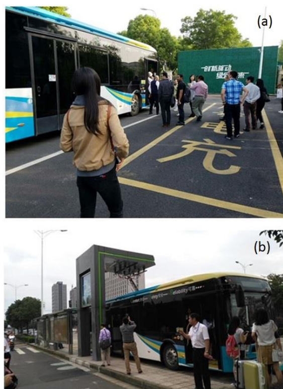
1 2 Figure 2: (a) Intra-city ride on an electric bus fully powered by supercapacitors (EDL capacitors) [9]. 3 (b) A supercapacitor bus is being charged at one of the stops along the bus route.
