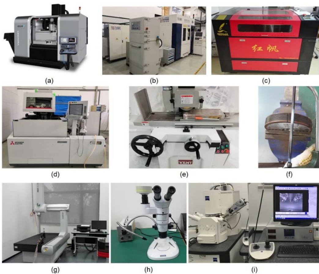
Figure 3.12 Experimental equipment. (a) 5-axis manufacturing centre; (b) Han's Nd: YAG laser machine; (c) Hongfan CO2 laser machine; (d) EDM; (e) grinder; (f) handsaw; (g) 3D coordinate measurement machine; (h) optical microscope; (i) SEM.
