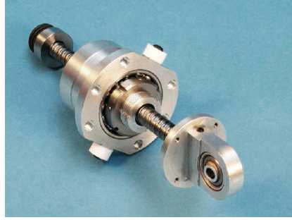
(a) Ball-screw inerter developed by Papageorgiou and Smith (2005) at Cambridge University
