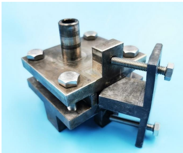
Figure 3.3. The mold used to orient CFs.
