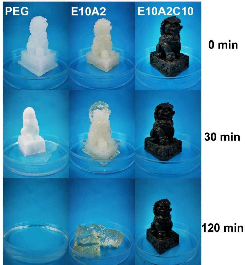
Figure 6.16. The molded lions made of PEG, E10A2 and E10A2C10 heated at 80 °C for different durations. The photos were taken at 0, 30 and 120 min, respectively.
