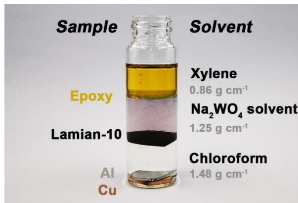
Figure 5.17. Samples flow in multilayer solvents with different densities.
