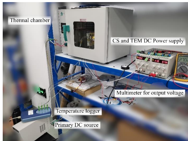
Figure 141 – Overview of the testing system.
