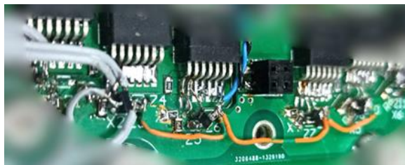
Figure 124 – Modified gate circuit (additional MOSFETs with capacitors)
