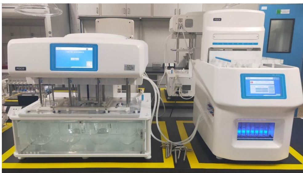
Figure 2.6 A dissolution tester with a sampling function, with a dissolution tester on the left and a sampling instrument on the right.
