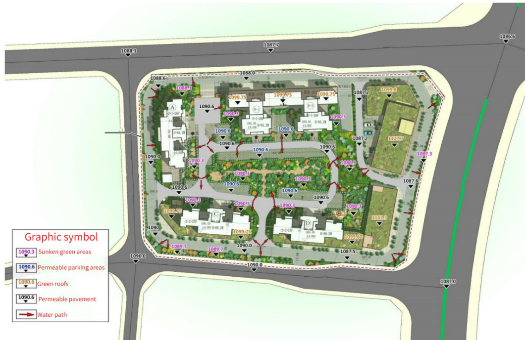
Figure 23 The layout of SCP facilities in a typical SCP community (Rui Da Jia Yuan)
