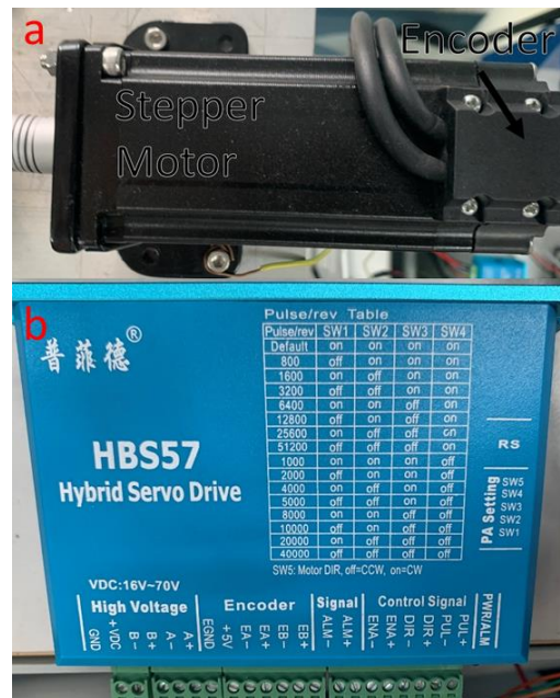
Figure 58. (a)57HSE3N stepper motor, (b) HBS57 stepper motor driver.
