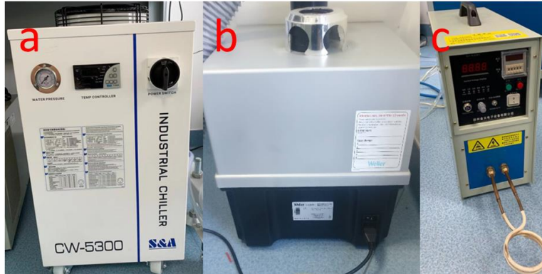
Figure 55. (a)Industrial chiller, (b)fume extractor, (c)ZVS induction heater.
