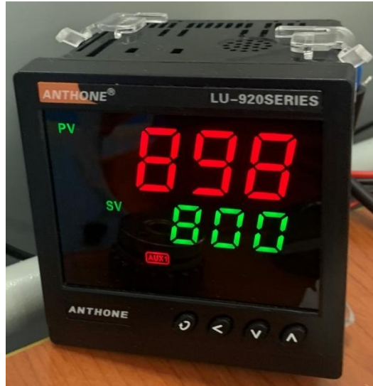
Figure 69. PID temperature control box.
